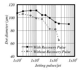
Figure 10. Dot diameter degradation by kogation
