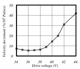
Figure 7. Kogation voltage characteristics.
