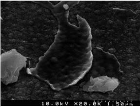
Figure 4. Kogation residues on heater surface.
