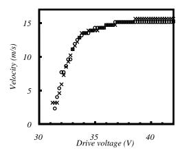
Figure 6. Drop velocity voltage characteristics.
