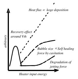
Figure 12. Conceptual kogation mechanism
