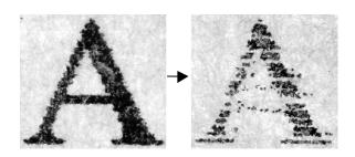
Figure 3. Print quality degradation by kogation.
